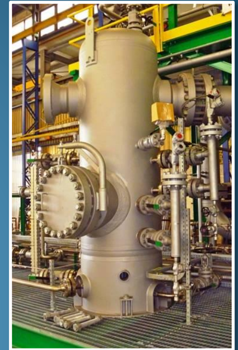
IN LINE SL TYPE - 45" # 1500 THK. 65 mm + 3 mm AISI 316L cladding
