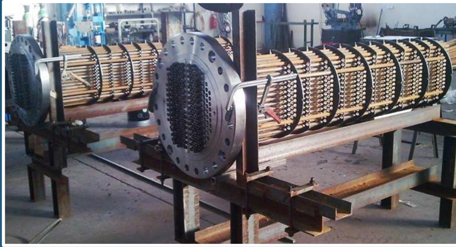
2 HEAT EXCHANGERS BEU TYPE – DUTY 1.500 KW # 600 each
