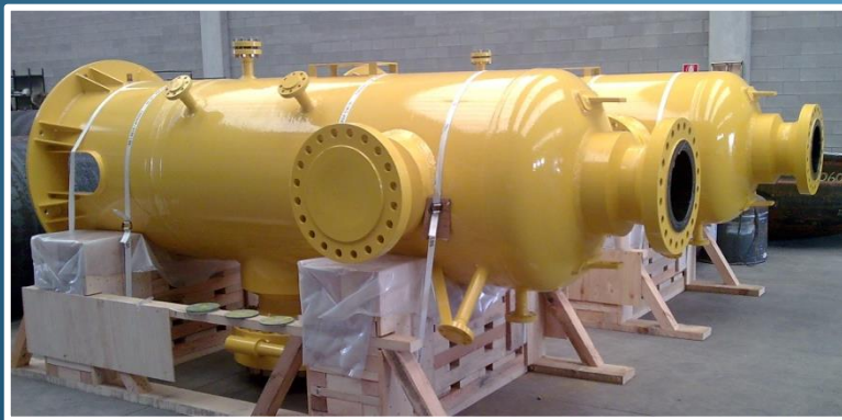
2 SC TYPE MULTITUBE SEPARATORS - 39" # 600
