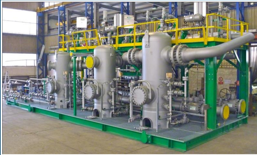
FIRST, SECOND AND THIRD STAGE SCRUBBERS PACKAGE FOR PROTECTION OF THE GAS COMPRESSOR
