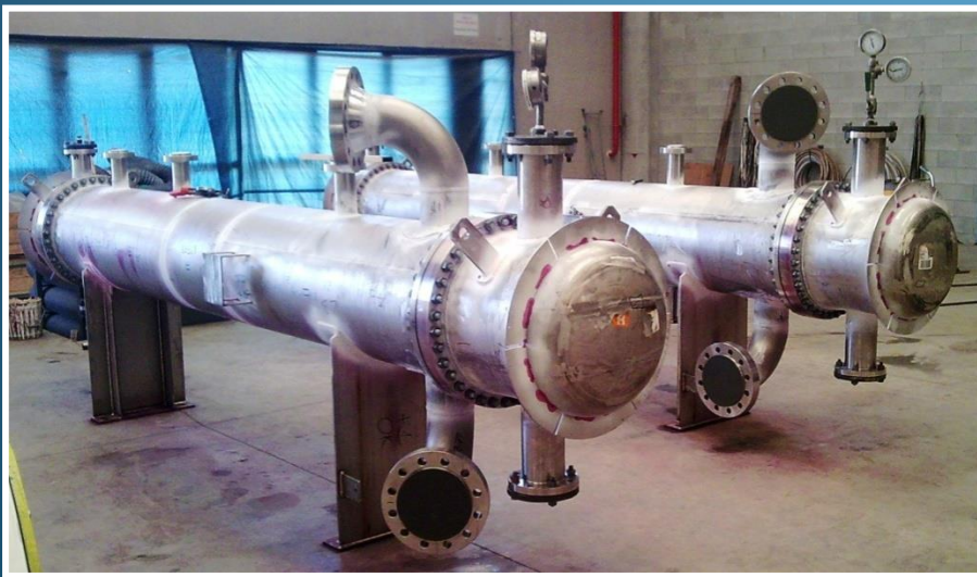
2 HEAT EXCHANGERS BFM TYPE – DUTY 787 KCAL/h # 600 each
