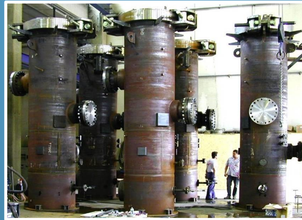
5 FILTER SEPARATORS SCF TYPE - 48" # 600
