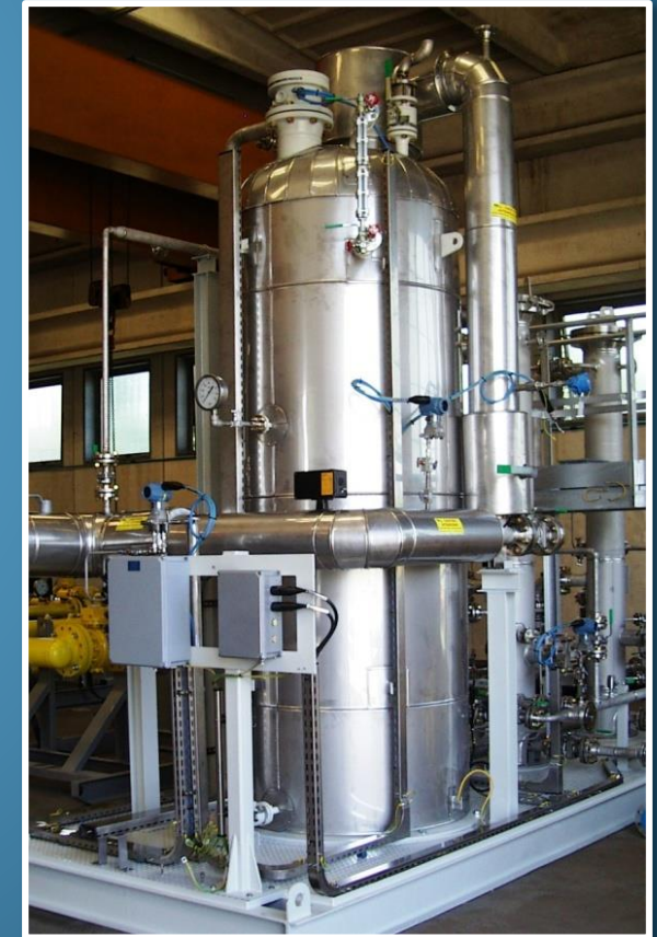
ELECTRIC HEATER RE TYPE - 125 KW # 300
