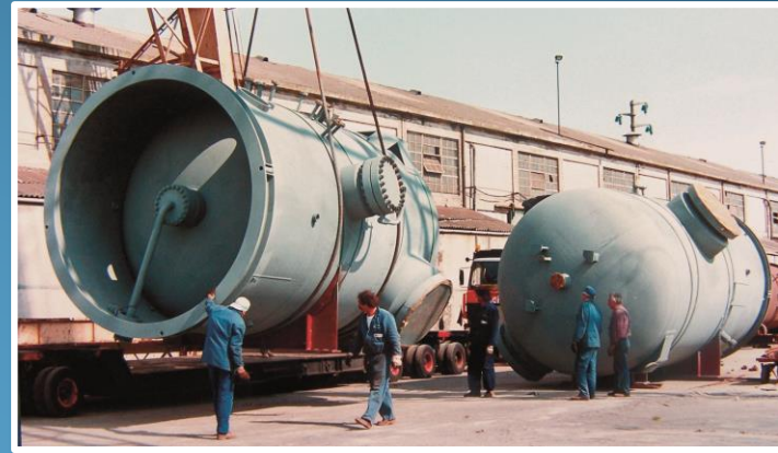
3 SC TYPE MULTITUBE SEPARATORS - 130" # 600 THK. 90 mm, 90 Ton each
