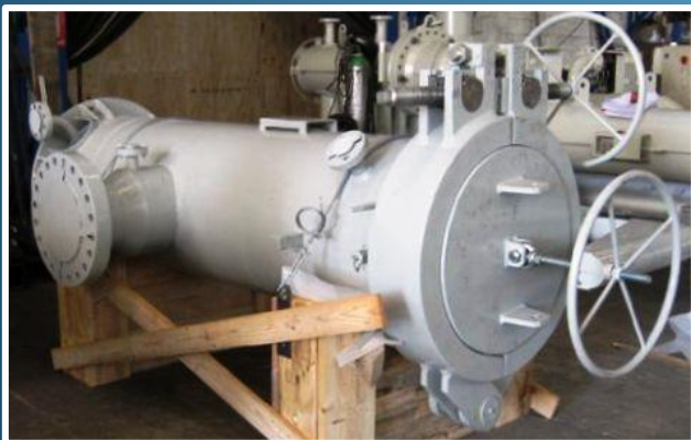
2 GAS FILTERS FCV TYPE - 32" # 900
